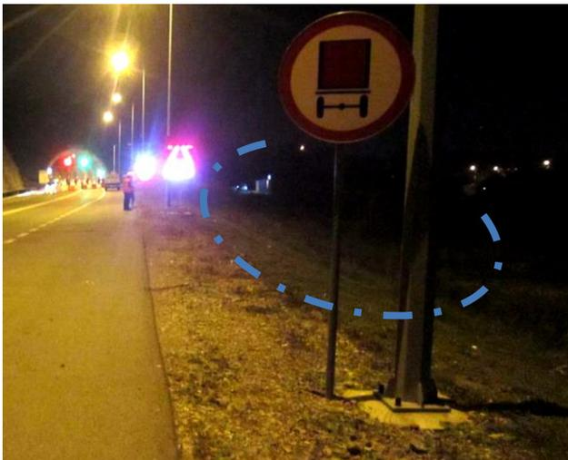
**Fig. 7** Unprotected lighting and road sign poles
