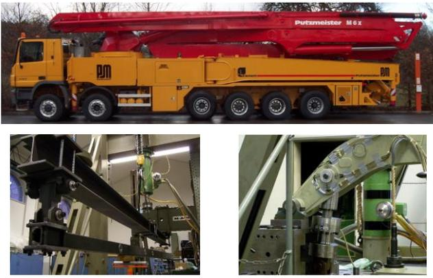
**Fig. 1** Mobile concrete boom pump 60-Meter-Class (Putzmeister AG) and test of parts of the boom
