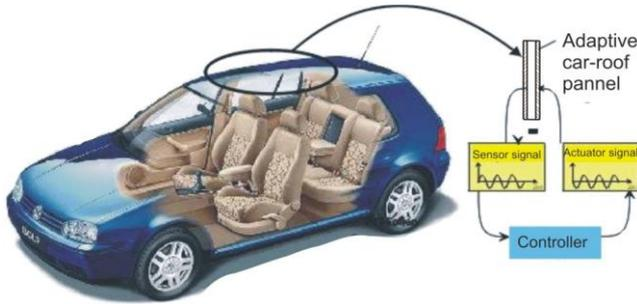
Fig. 8 Adaptive car roof for cabin noise reduction
