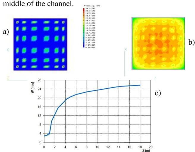
Fig. 3 Particles of flour: a) position of particles, b) velocity in cross-section c) velocity along the channel
