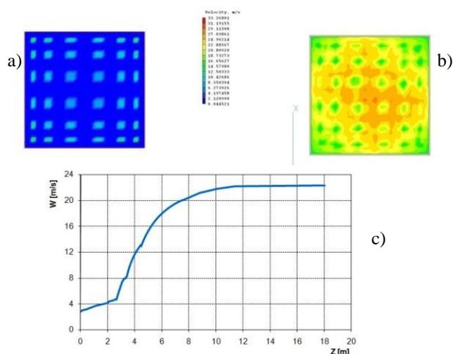
Fig. 4 Particles of quartz a) position of particles, b) velocity in cross-section, c) velocity along the channel
