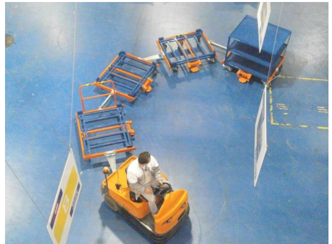
Fig. 3 Tugging trains composition with working aisle
