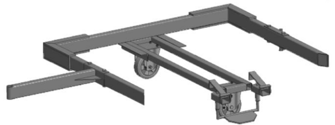
Fig. 4 Trailer (E – frame) of mechanical tugging train [6]
