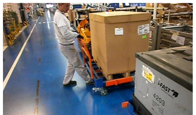
Fig. 6 Loading/unloading operation with foot pedal
