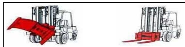
Fig. 1 A forklift with a gripping tool in a shape of spoon and in a shape of fork
