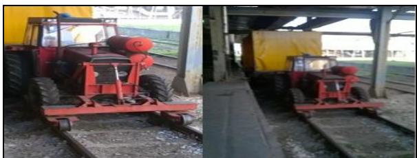
Fig. 2 Loco-tractor for the transport of railway wagons in internal transport
