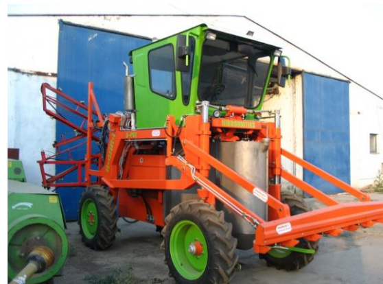
Fig. 2 Self-propelled agricultural machine made by Hidromatik, Serbia. Windshield is inclined towards outside, the roof is white. Further improvement in heat gain reduction can be achieved by longer roof overhang, adjustable sun visors and solar reflective glazing
