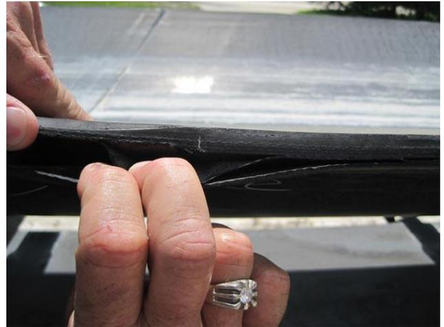
Fig. 2 Edge delamination at rubber conveyor belts
