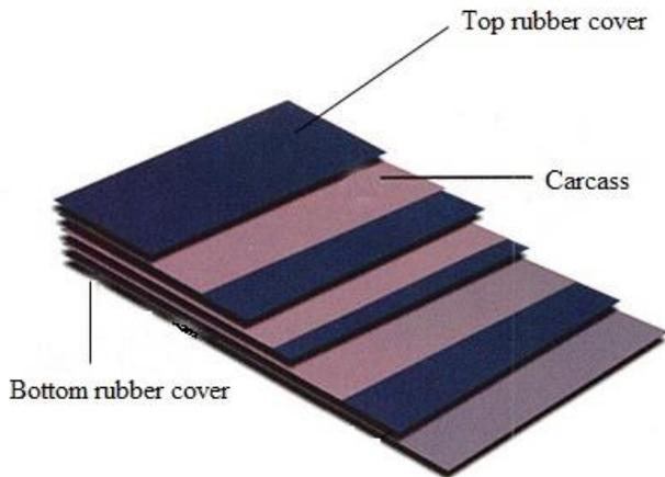
Fig. 1 Layers in rubber conveyor belt with carcass
