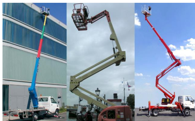
Fig. 1 MEWP boom types: telescopic, articulating and combined boom type
