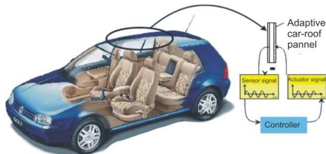
**Fig. 1** An example of a smart structure – car roof with active elements for noise reduction
