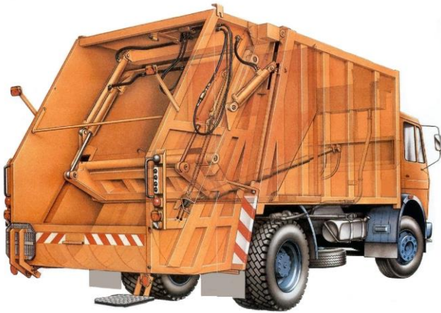
Fig. 3 Refuse vehicles with a powerpress system
