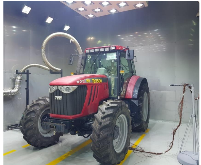
Fig. 2. Farm tractor in environmental chamber during the experiments carried out by Oh et al. [12]
