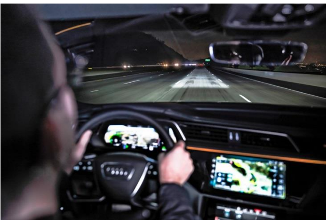
Fig. 6 Marking the distance from the vehicel in front of LED Matrix Headlight (source: https://www.carmagazine.co.uk/ )
