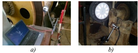
Fig. 21 Measuring places: a) the incremental encoder connected with the measuring wheel positioned on the rim of the brake disc, b) the optical sensor (number of revolutions sensor) positioned on the cage
