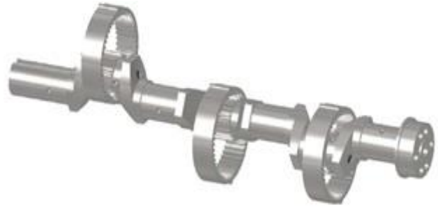
Fig. 2 The crankshaft of the engine with three pistons
