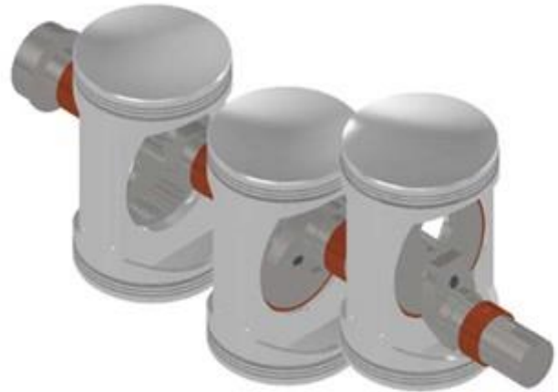
Fig. 3 The crankshaft of the engine with three pistons
