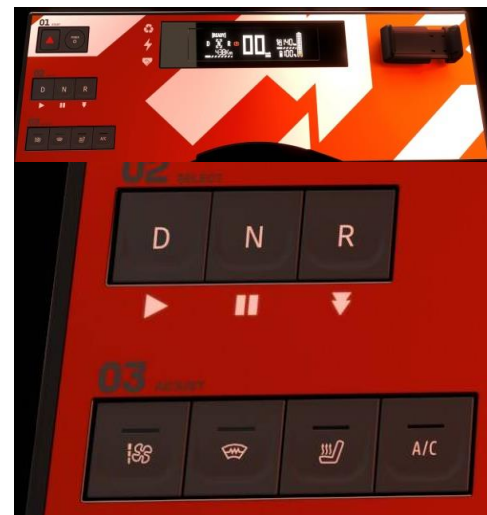
Fig. 3 Control panel of a microcar equipped with the HVAC: commands of blower, windshield heater, seat heating and AC (Mobilize Duo) [18]
