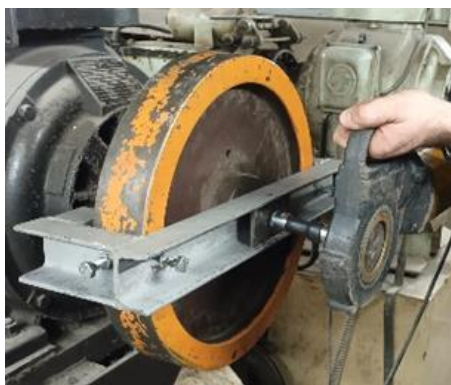
Fig. 7 Measuring lever mounted on the flywheel of the electric motor
